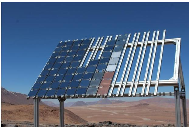
As it is being proved that standard tests are not able to reproduce the degradation adequately, an improved testing methodology is being developed within the project. The in-service degradation is analysed based on an extensive outdoor campaign and at the same time advanced test procedures are investigated. For the outdoor campaign small mirror samples of different types
