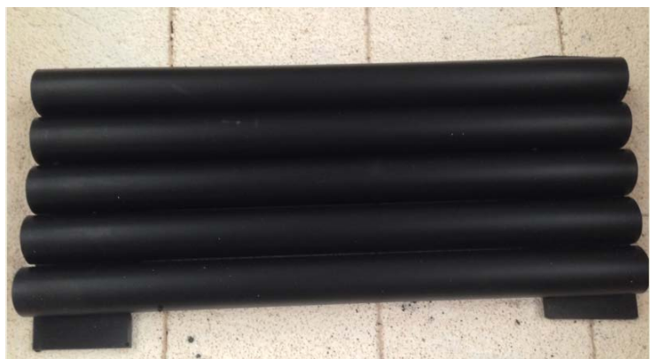
Coating BrightSource pipes
